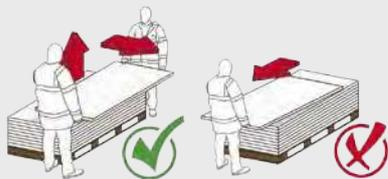
Boards should always be lifted by 2 people and not dragged across each other to prevent un-necessary scratching or damage
