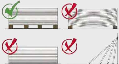
Resistant boards should be stored flat, raised from the ground on a pallet, in dry conditions indoors and be under cover. Boards should not be leant upright for long periods of time
