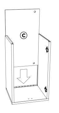
6 Press end panel A into top/bottom panels B and gently tap with a mallet
