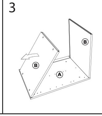
Press end panel A into top/bottom panels B and gently tap with a mallett
