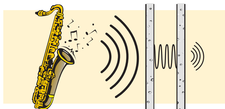
Lightweight constructions outperform the acoustic damping of massive walls.
